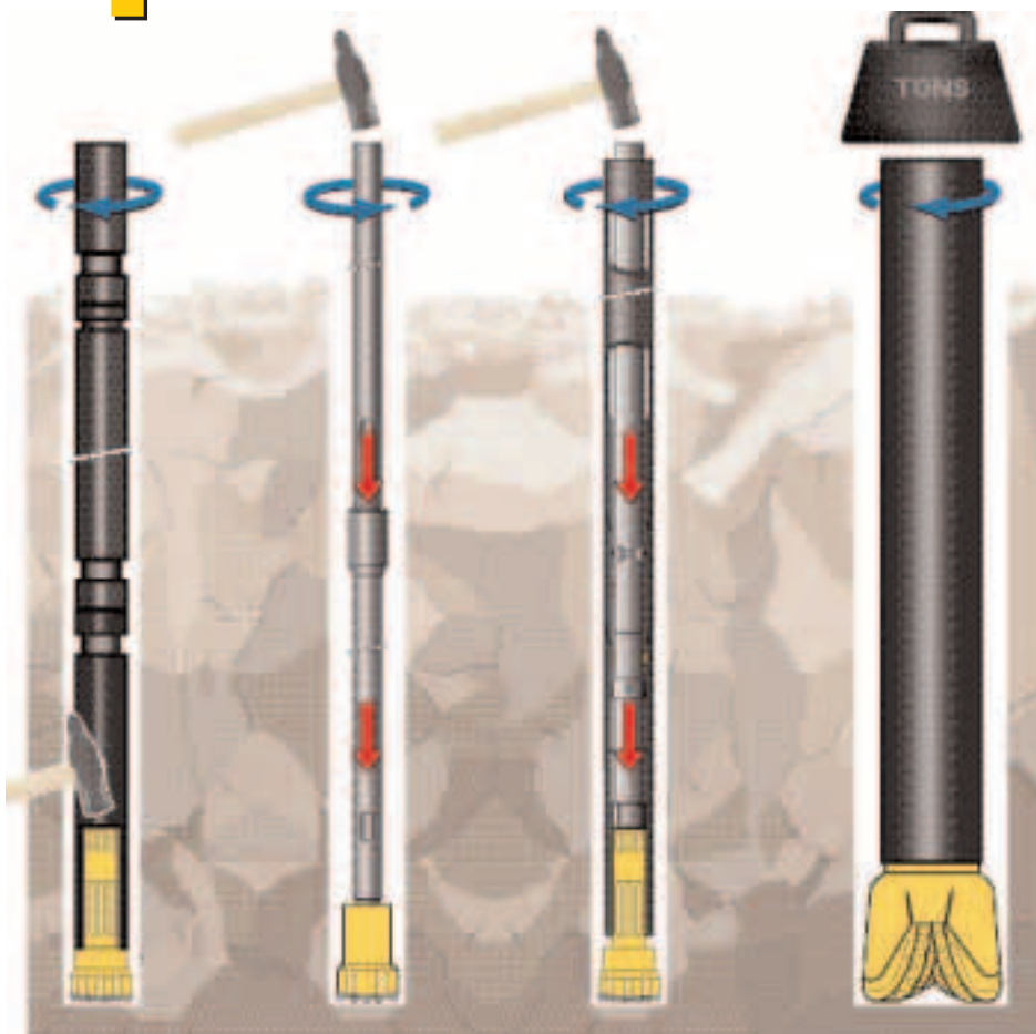
Fig 1. Drilling methods (1) Down-the-Hole (DTH); (2) Tophammer; (3) COPROD; (4) Rotary tricone.
